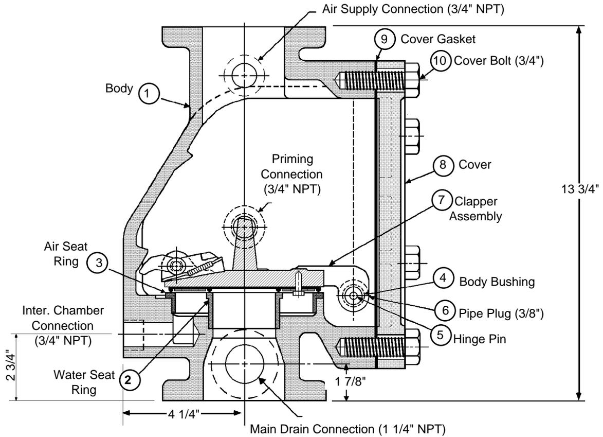
**Note: The Clapper Assembly may be removed from the body of the Dry Pipe Valve by removing the two 3/8" plugs (#6) and removing the hinge pin (#5).**
